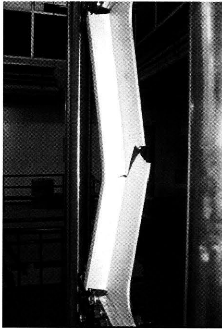
Figure 3-57: Side view of the final stage of the SSDENT specimen where the final deformation is observed
