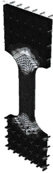
Figure 4-6: Boundary conditions imposed to the "dogbone" specimen at the numerical simulation. Note that the degree of freedom in the loading direction is released on the top of the specimen
