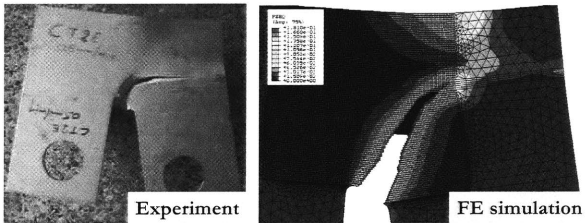
Figure 4-25: Comparison between the crack pattern obtained from the experiment (left) and the numerical simulation (right) for the T-type extruded CT specimen
