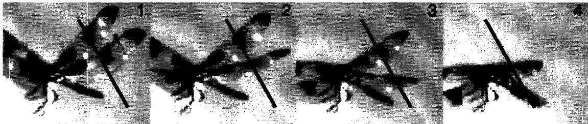
Figure 2. High speed camera images of the dragonfly wing path for hovering. Note both the horizontal and vertical components of the wing path. (3)
