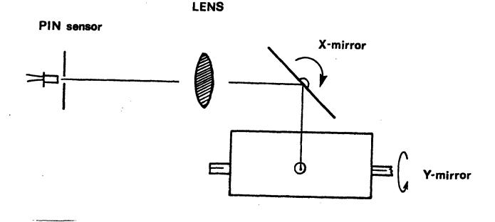
The currents to drive the mirrors comes from a pair of scanner controllers which receive their input voltages from digital-toanalog converters whose digital input is supplied by the program. There also exists a second set of drivers attached to a smaller mirror deflection system which is rigidly attached to a helium neon laser. By placing the
