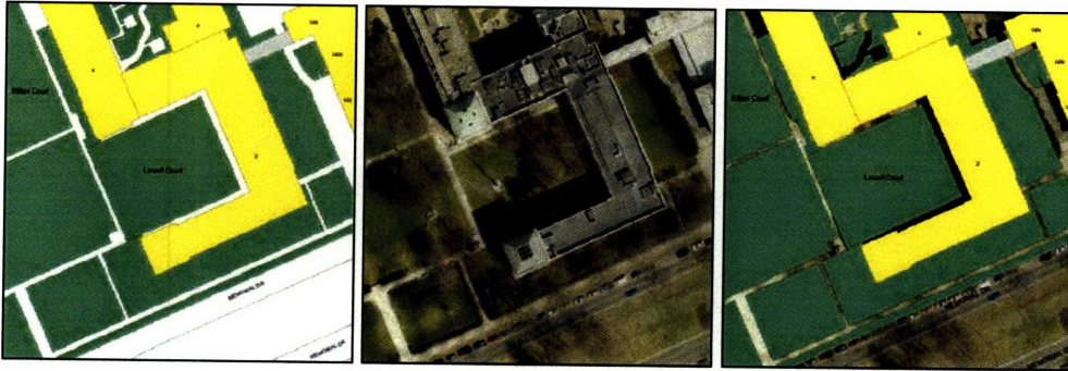
Figure 3-17: Three layers of the same “231232” image tile – type “m” (left), type “a” (middle), type “h” (right)
