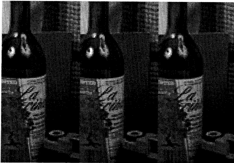
Figure 4.2: Effect of linear distortion on the Highs component. From left to right: original, Butterworth 3rd order, Butterworth 11th order. B^+ = F_s .
