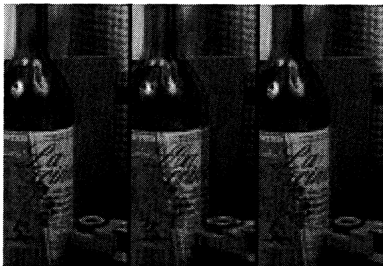
Figure 4.3: Effect of linear distortion on the four by four subbands issued from the Highs component. From left to right: Butterworth 3rd order, Butterworth 11th order, approximation of an ideal low-pass filter. B^+ = F_s .
