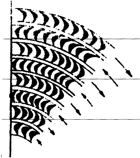
Figure 4-2: Diagram of the Ljungstream steam turbine; the two rows of blades comprising each of the stages rotate in opposite directions so that they can be both regarded as rotors, Figure accepted from [7].
