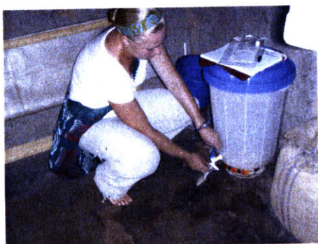
Figure 14: Taking filtered water sample from a KOSIM water filter (photo: Amin Hussein)
