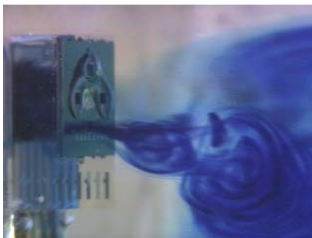
Figure 2.6: Side view of device showing release of methylene blue into a solution upon activation.
