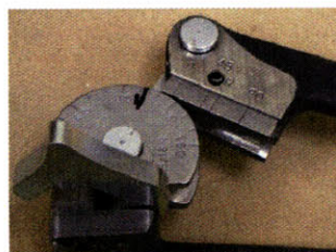
(a) Standard bending tool for 90° bend (OD 3/8”, R 15/16)
