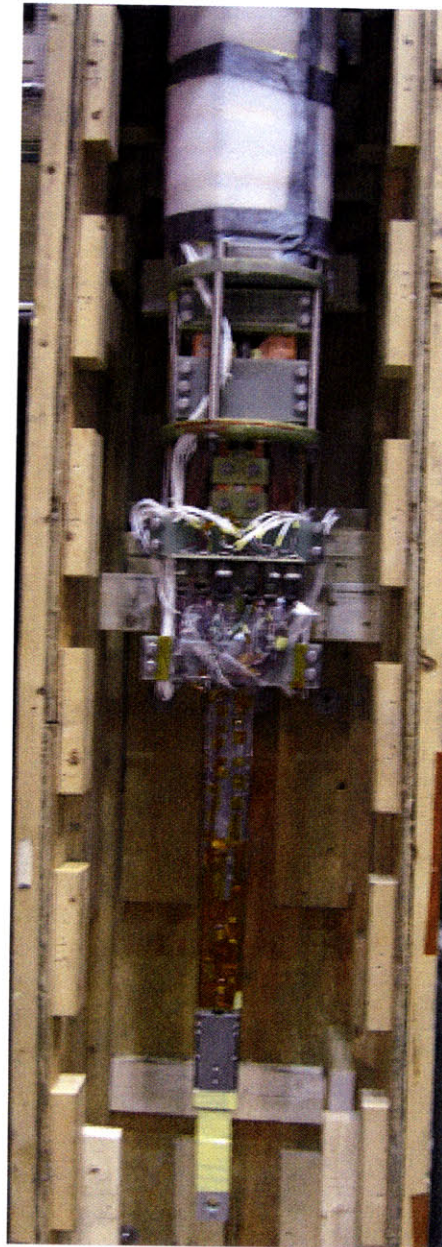
Fig. I.26 Probe ready to be inserted into the dewar.
