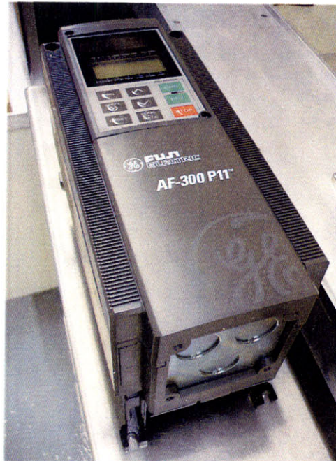
Figure 11: VFD control (Model Fuji Electric AF-300 P11).
