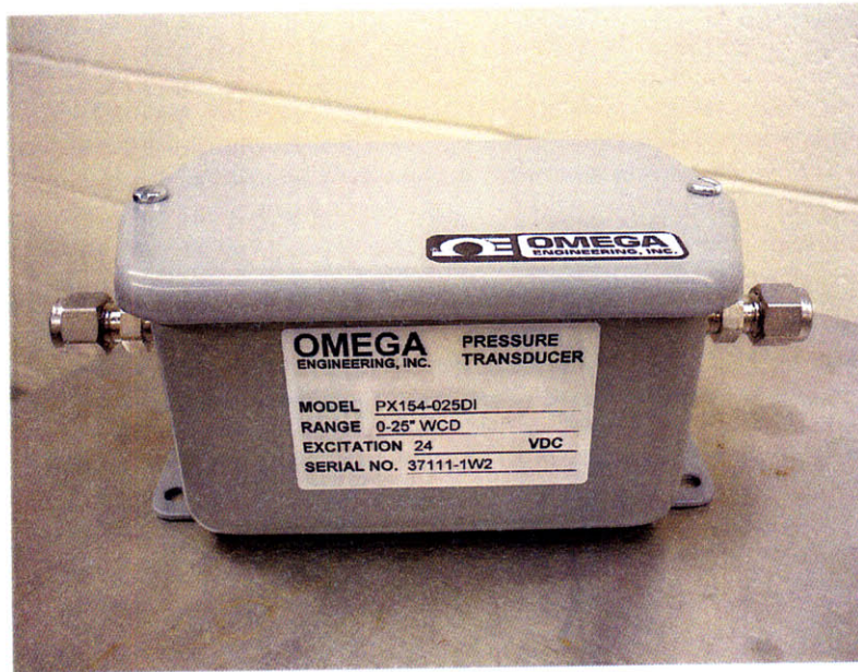
Figure 20: Low-range differential pressure transmitter PX154-025DI.
