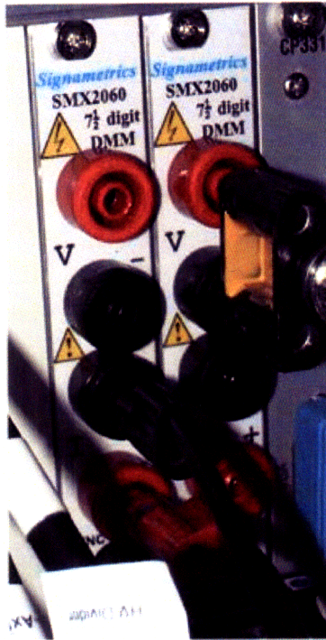
Figure 3- 4: Signametrics Card Inputs. The DMM card on the left has connectors in the current terminals for measuring the beam current. The DMM card on the right has connectors in the voltage terminals for measuring the beam voltage. Both cards are installed on the PXI computer.
