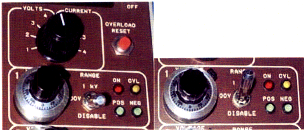
Figure A- 1: Suppressor high voltage supply switch. The switch must be moved from “Disable” to “1 kV” in order to activate the secondary electron suppression mechanism of the Faraday Cup. The range dial adjusts the voltage bias on the suppressor, but in order to see the voltage on the digital readout, the upper knob must be turned to the appropriate channel.
