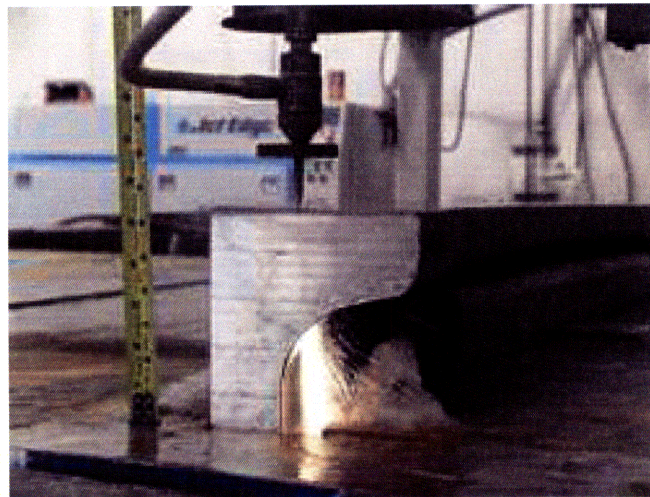
Figure 38 Water jet cutting through solid titanium [9]
