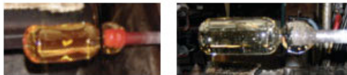
Figure 8. The left picture was taken while the piece was hot and moving. The right picture shows the piece when very cold relative to the left picture. Pictures are of a solid piece used for torque measurements.
