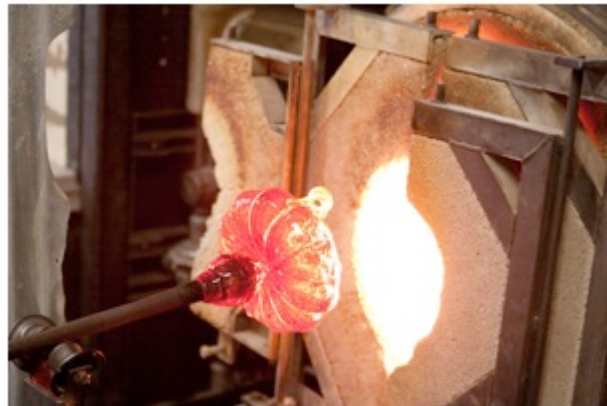
Figure 10. Pumpkin in front of glory hole with blowpipe resting on yoke.
