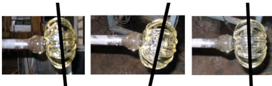
Figure 8. The left picture was taken while the piece was hot and moving. The right picture shows the piece when very cold relative to the left picture. Pictures are of a solid piece used for torque measurements.
