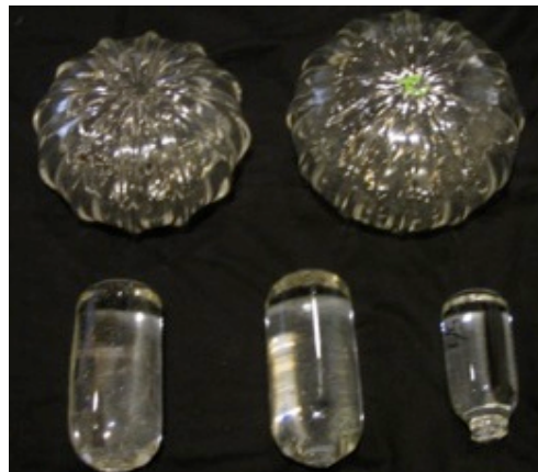
Figure 19. Picture of samples used for torque testing. Ellipsoid with optics ridges, (pumpkin bodies), on top and solid cylinders on bottom.
