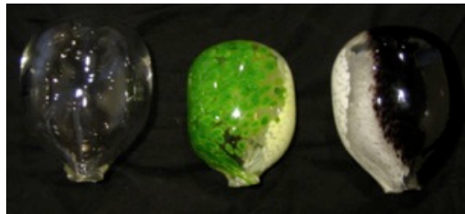
Figure 18. Picture of annealed samples from dynamic temperature tests with color.
