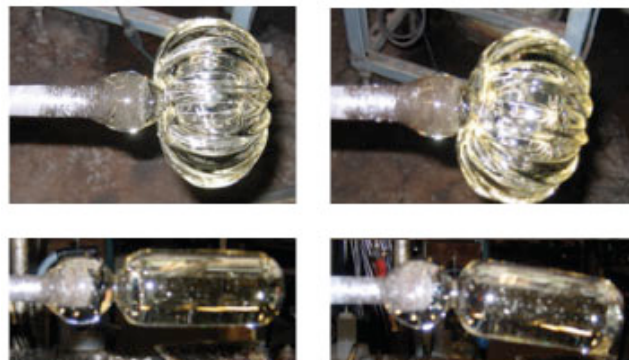
Figure 20. Pictures of pumpkin body and solid cylinders used for torque testing. Left hand images are on center and right hand images are off center.
