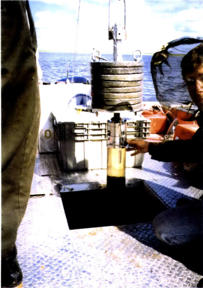
Fig. 30. "Ob Venture" Sediment coring in progress. Expedition "Ob Estuary - 1994".
