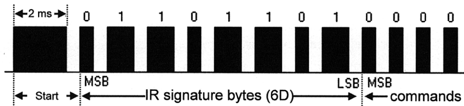
Figure 4.12 A standard IR packet in our protocol.
