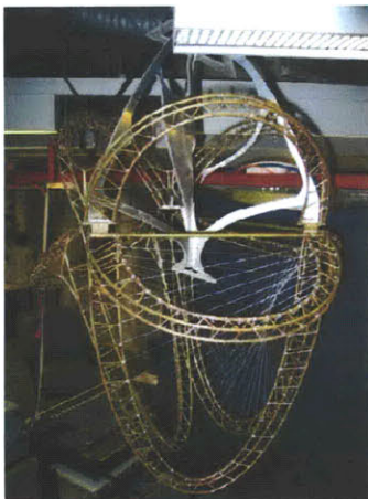
Figure 23: Quarter-scale Chandelier model This more recent model has the wings oriented downward so that they can enclose Evvy.
