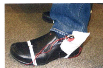
Figure 68: James Maddalena wearing sensors Opera singer James Maddalena performed during test capture sessions wearing two arm sensor assemblies, breath sensor, and shoe pressure sensors.
