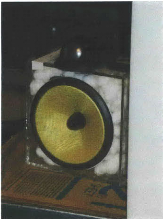
Figure 45: Wall speaker cluster These mid-range and tweeter clusters were positioned behind the acoustically transparent screen for the sound spatialization tests of the wall prototype.
