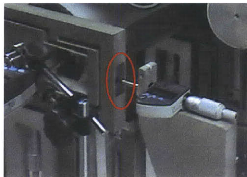
Figure 62: Stainless Steel Surface Attached to the Flexure to Avoid Permanent Deformation.
