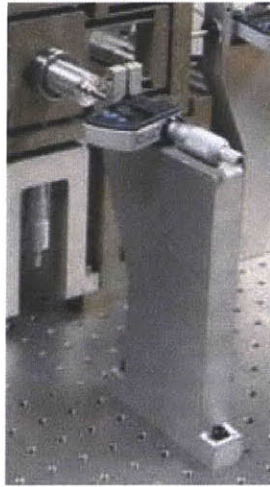
Figure 54: Central Fixture; the Micrometer Head Supported by this Fixture Adjusts the Position of the Print Roller along X.
