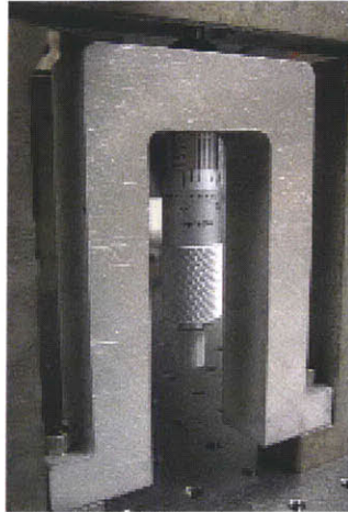
Figure 52: One of the Two Vertical Fixtures Assembled in the Frontal Flexure.
