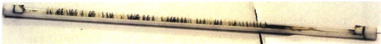
Figure 13: Small Autoclave Loaded Sample Train
