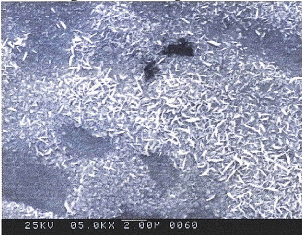
SEM Image at 5000x of the Light Oxide
