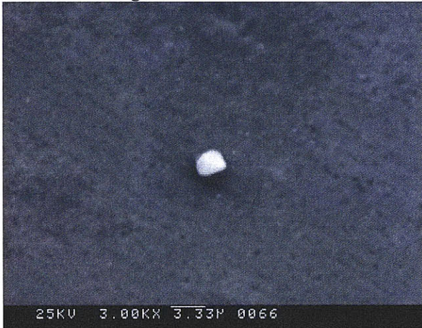
SEM Image at 3000x of an Al-Ni-Cr Precipitate
