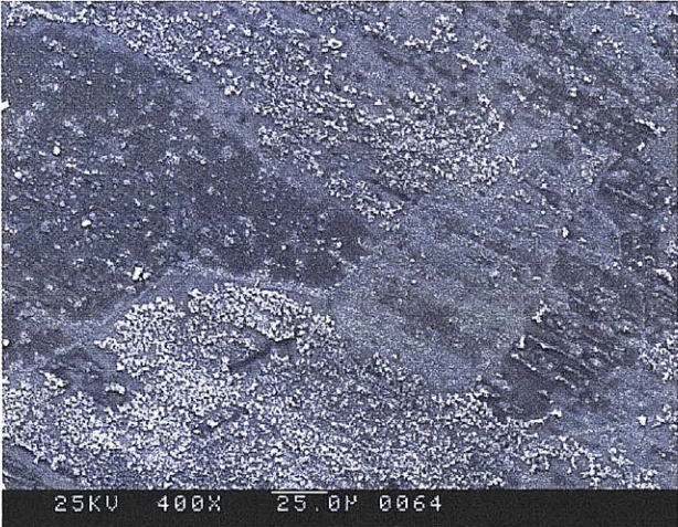
SEM Image at 400x of the Light and Dark Oxide
