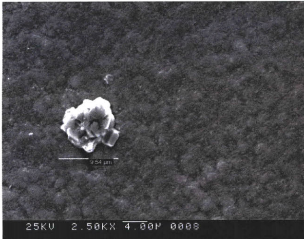
SEM Image at 2500x of Titanium Precipitate
