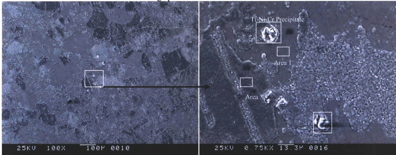
SEM Image at 100x of the General Surface Morphology
