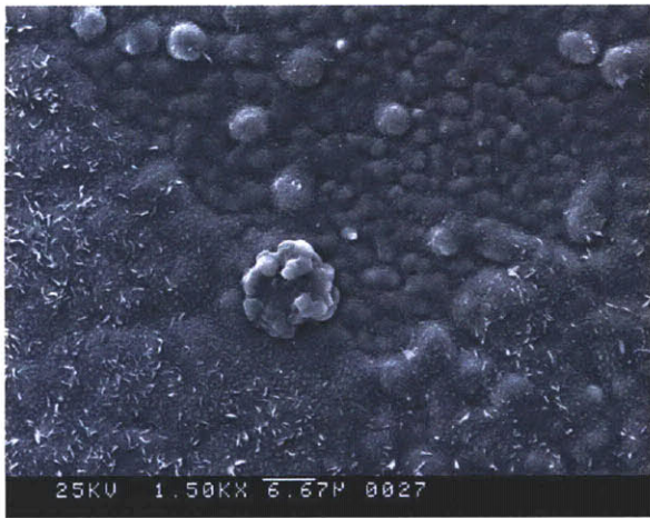
SEM Image at 1500x of Titanium Precipitate
