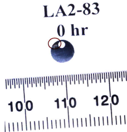
Figure 8: LA2 Series Sample with Plastic Deformation on the Opposite Side of the Etch
