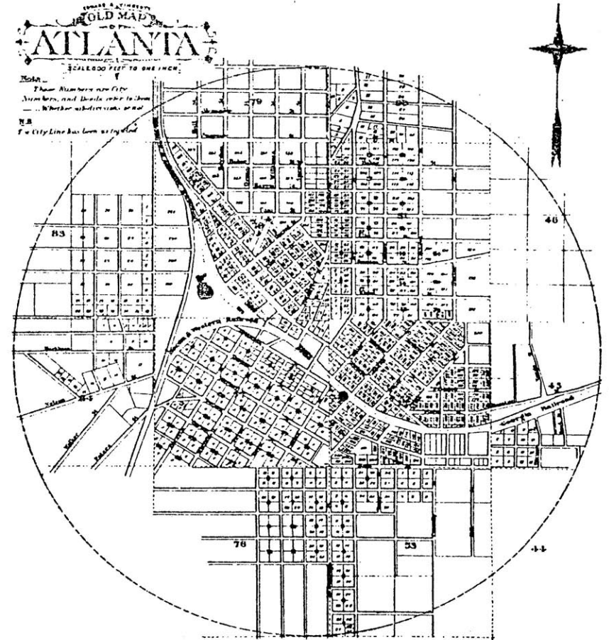
Figure 9.35 - Atlanta, plan of the central part of the city in 1847 within a circle of a radius of one mile. The plan shows how the early unrelated gridiron districts of the first railway settlement were subsequently resolved into a standard north-south, east-west orientated pattern.
