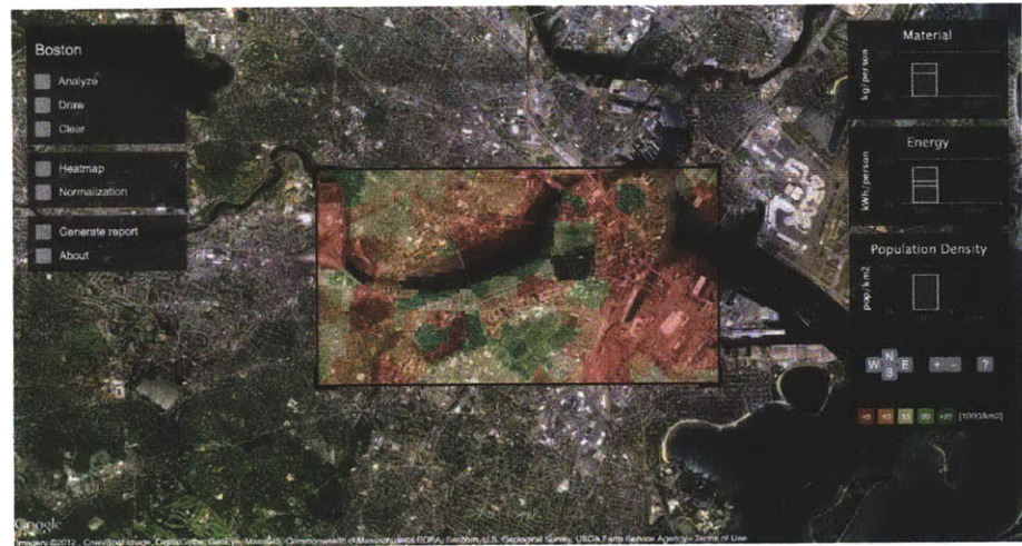
Figure 7.6: Neighborhood Visualizer v0.9 (April 2012) . The user can choose between three different heatmap options to overlay a population density measure, an energy measure or a material measure. The term heatmap was used as a colloquial term to describe the raster overlay.
