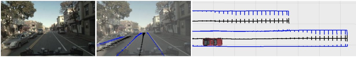
Fig. 10 (left) The farthest boundary of the opposite lane is occluded by other vehicles. However, by maintaining a joint distribution over centerline geometry and lane width, (middle) the system can still maintain an estimate of the opposite lane, using observations of the closer boundary. (right) A synthesized overhead view of the vehicle and its lane estimates. Black curves correspond to the estimated lane centerlines, and blue curves denote the marginal distributions of the lane boundaries. Short line segments extending laterally from the curves indicate control point uncertainty.
