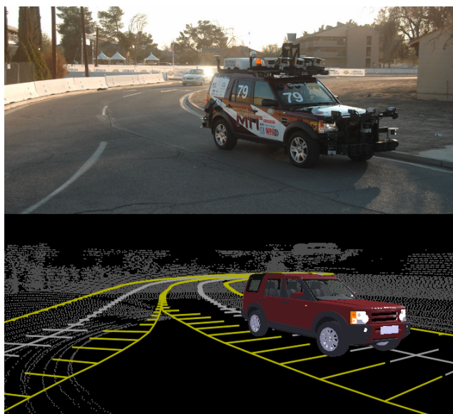
Fig. 1 (top) MIT's autonomous vehicle. (bottom) Lane estimates; uncertainty indicated by short perpendicular lines.
