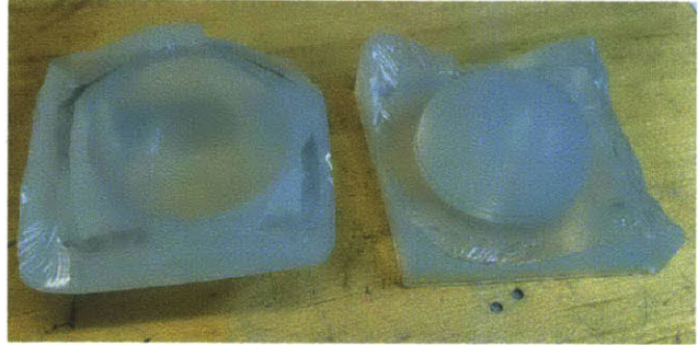
Figure 50 Small test mold split
