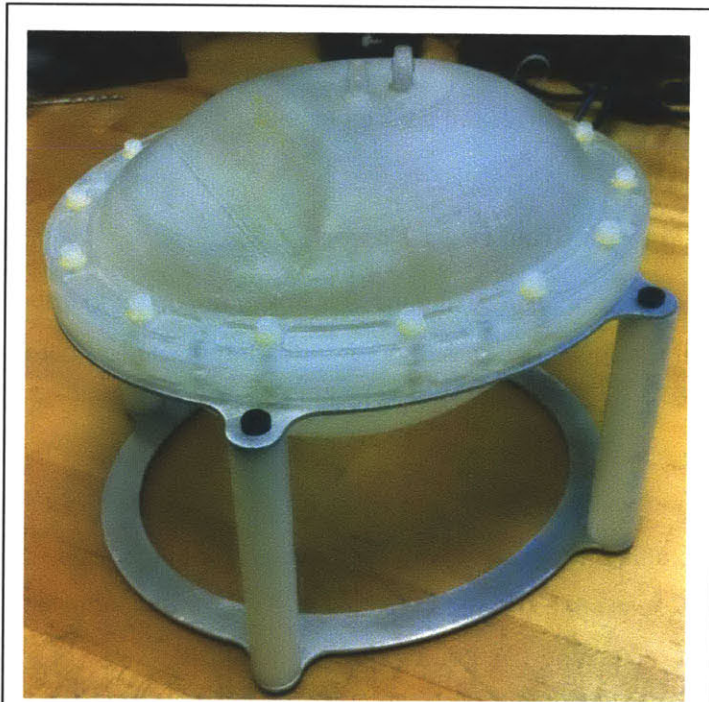
Figure 24 Holder and holder stand (used for assembly, degassing, storage)
