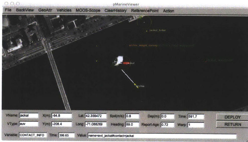
Figure 5-7: Moving Target at t=5 : The cluster of particles eventually consolidate to the contact's location.
