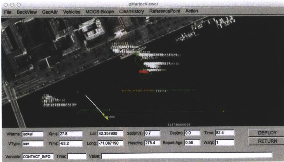
Figure 5-5: Moving Target at t=3 : Particles begin to form cluster with similar relative motion as a result of the resampling subroutine transforming the particle distribution by drawing with replacement from the previous distribution.
