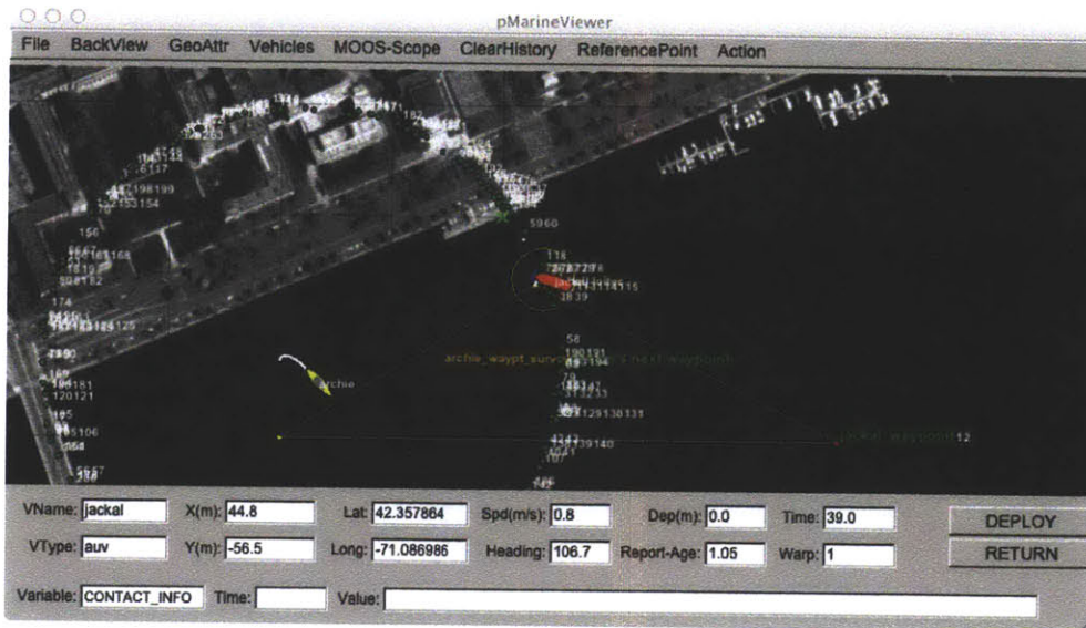
Figure 5-3: Moving Target at t=1 : Once ownership received range information, initialization of particles occur along that radius.
