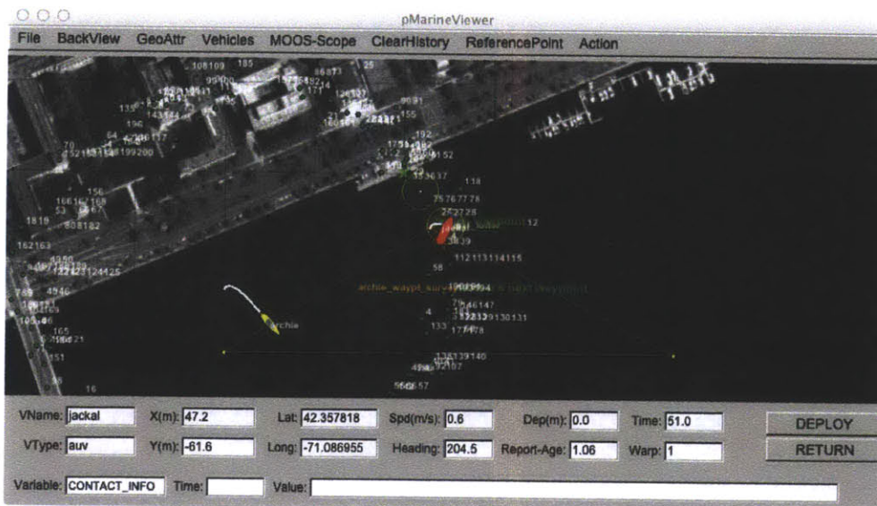
Figure 5-4: Moving Target at t=2 : Particle separation begins as a result of each particle being initialized with different courses and different speeds.
