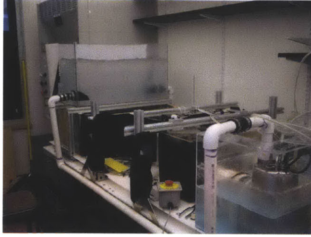
Figure A-2: Photo of the water-tunnel hardware. The upper left shows the settling tank filled of water as it is fed by the stainless steel pump. Note the black fabric used to prevent any unwanted reflections of the laser sheet back into the lab.
