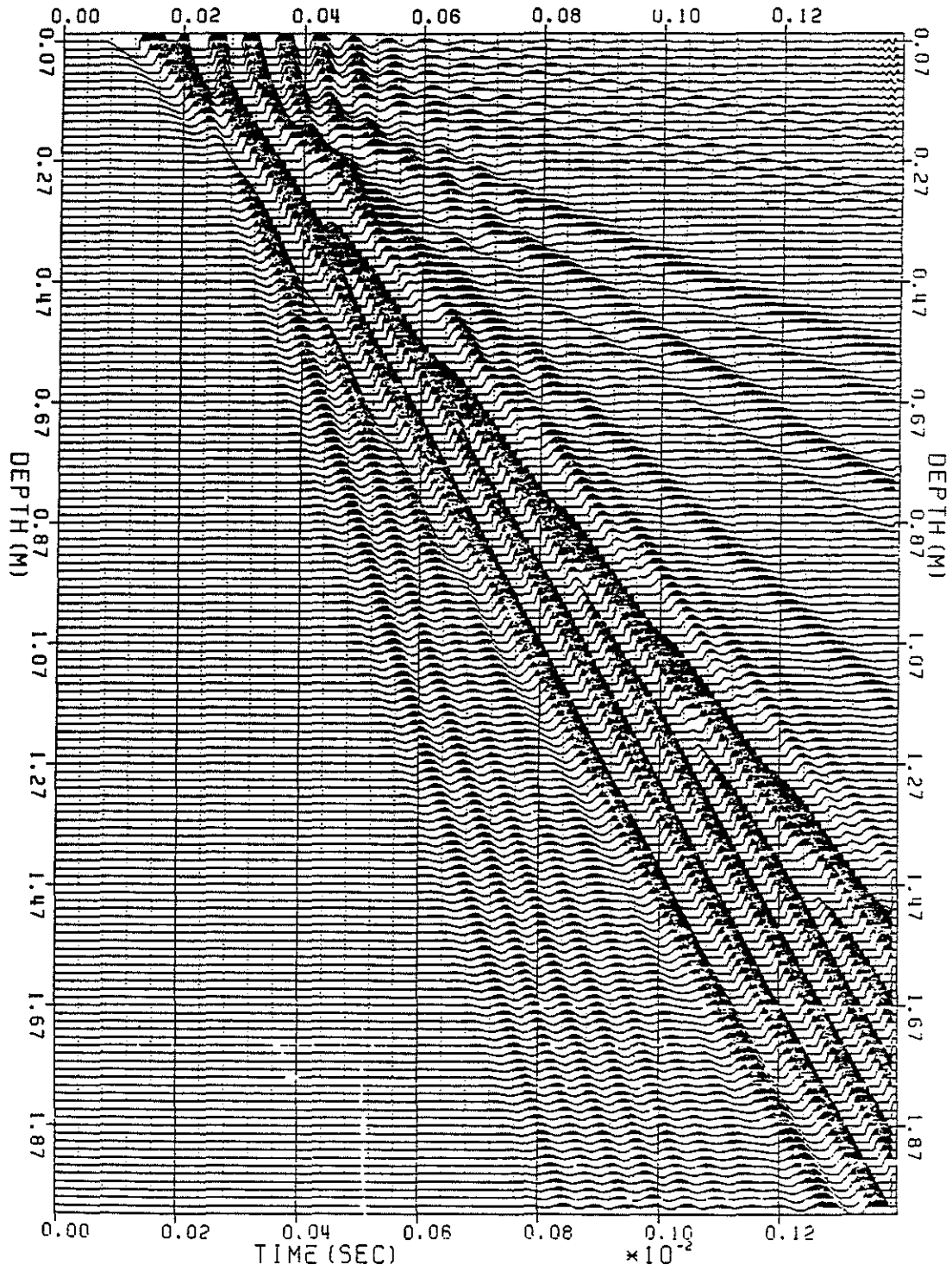
Figure 14. FD synthetic microseismogram using Model 2 in a damaged zone with a rigid tool.
