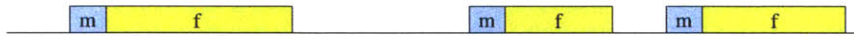
Figure 2-3: The use of idle fill characters is not allowed in bursty transmission. Hence, the time between two packets is silent.
