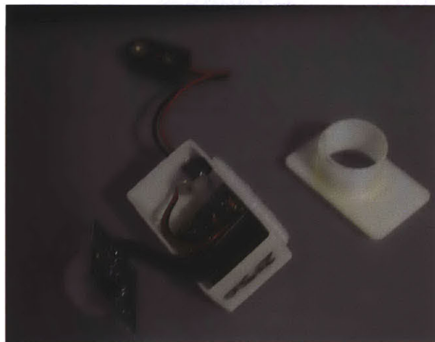
(b) PIR disassembled
