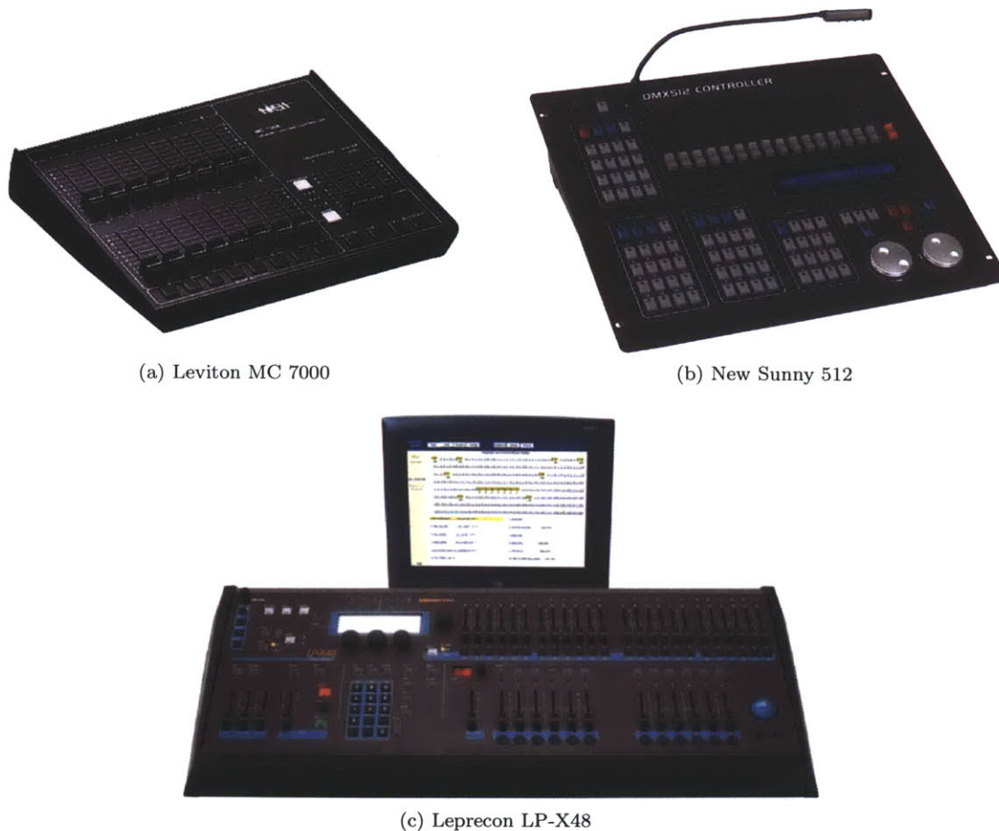
Figure 2.2: Three examples of physical DMX control consoles from the theatrical lighting community. They are arranged in ascending order of complexity though the modalities of interaction is largely the same: the button, the slider, the switch, and the knob. These controllers are incredibly generic in their controls but this becomes a barrier to entry for the average user.
