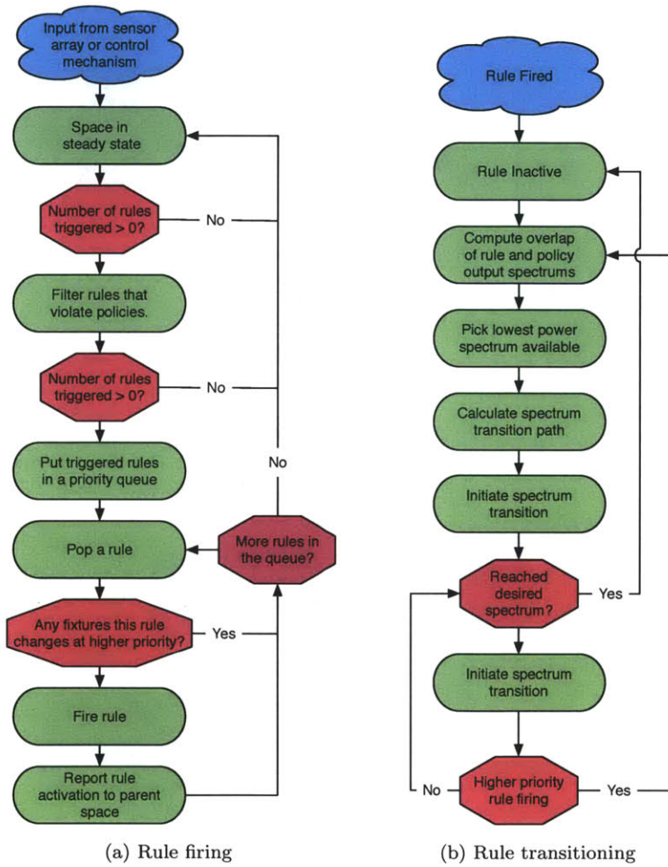
Figure 3.7: Flow charts diagramming the ways a space determines if a rule can fire and actions taken by each fixture to influence transitions.
