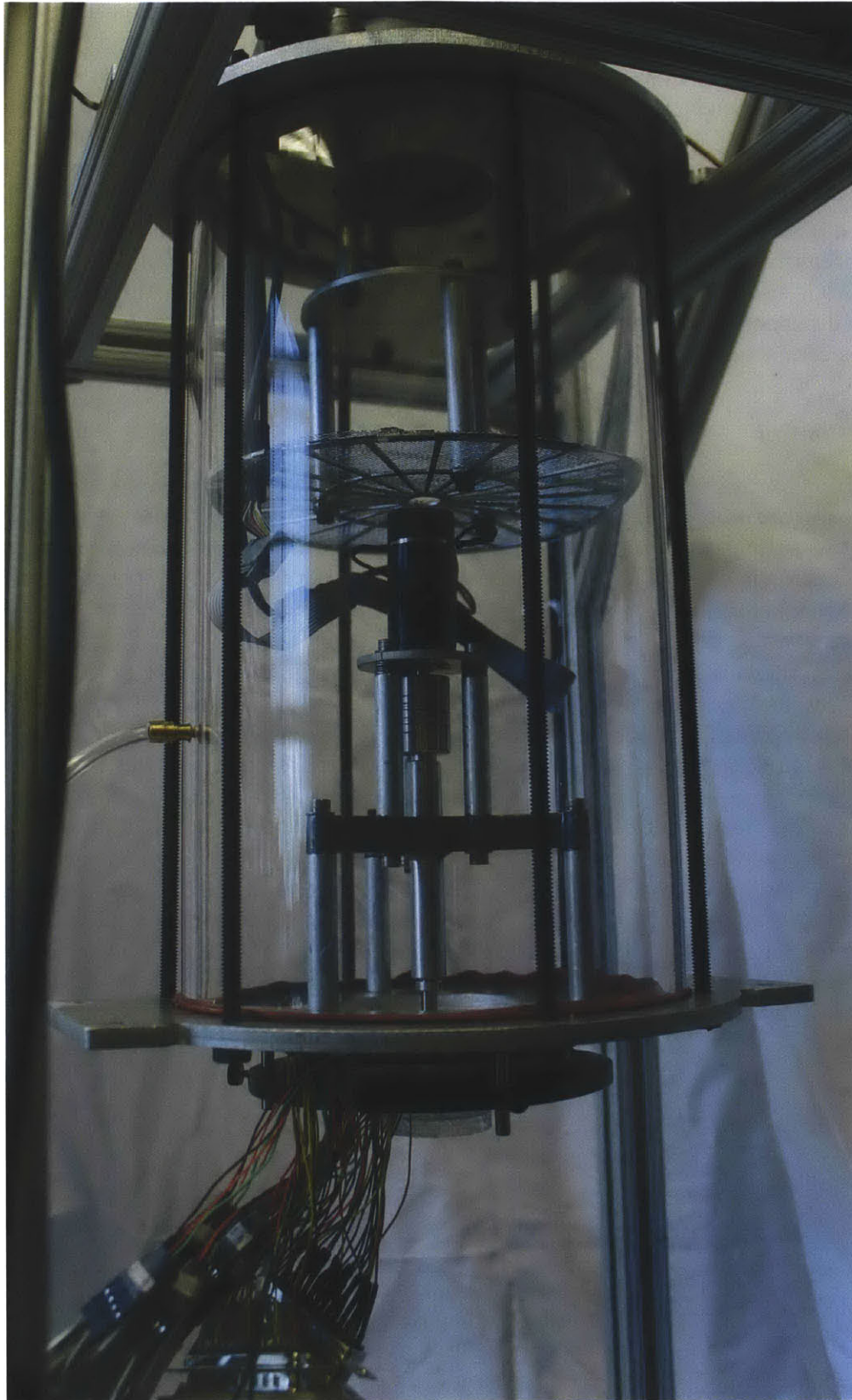
Figure 2-12: A photograph of the plenum section, showing the location of the upstream total pressure tap.
