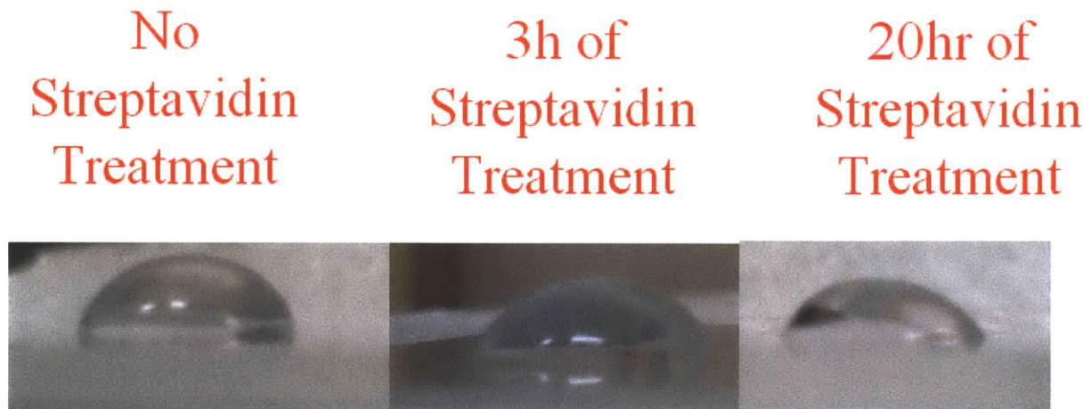
Figure 15: Biotin is an extremely hydrophobic molecule with a water contact angle approaching 90 degrees. Streptavidin is highly hydrophilic with a water contact angle nearing 180 degrees. The water contact angle is increasing with exposure time of streptavidin, illustrating that the surface is indeed being coated with streptavidin.
