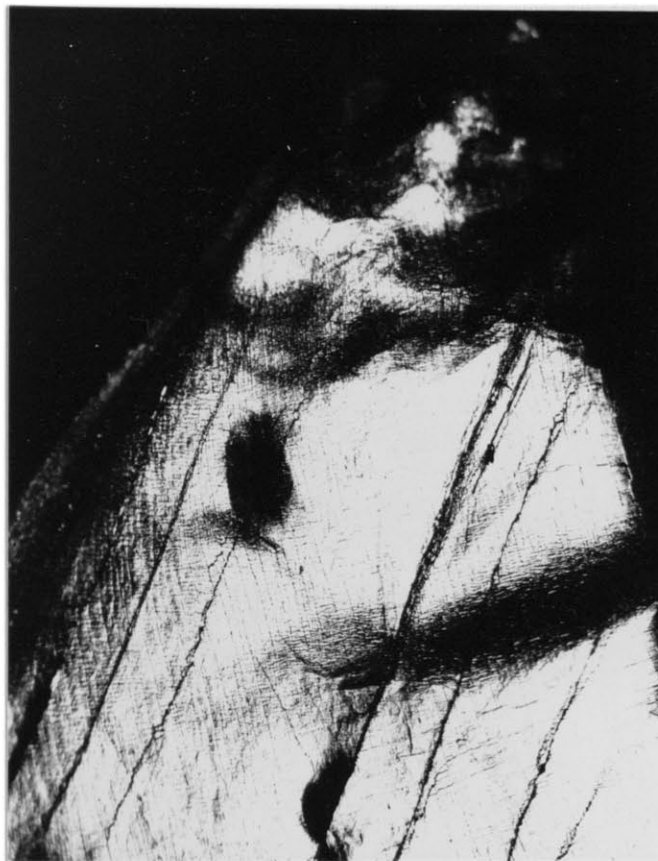
Figure 47. (Specimen P-10). 30.4 hours after reaching 1100^{\circ} F, fractured. Non-homogeneous deformation occurred at the region close to the right edge of the specimen and the heavily slipped band. 50 X.
