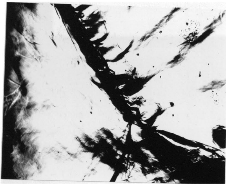
Figure 64. (Specimen P-6). Deformation bands started from that part of grain boundary where sharp curvature occurred as a result of uneven boundary sliding and migration. 100 X.
