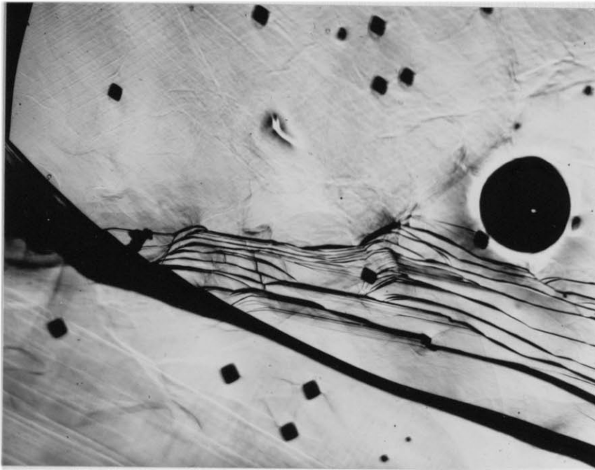
Figure 14. (Specimen P - 8, front surface). Uneven nature of grain boundary sliding and migration. 100 X.
