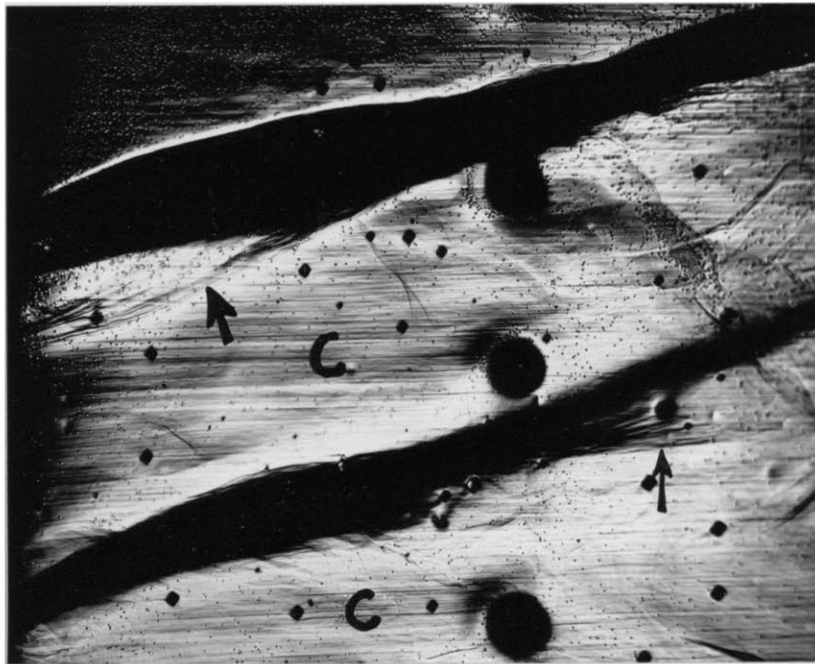
Figure 50. (Specimen P-8, front surface). Effect of grain boundary on the development of slip bands. The upper band was fully developed, the lower band not. The arrows indicate the regions where cross slip has taken place. 50 X.
