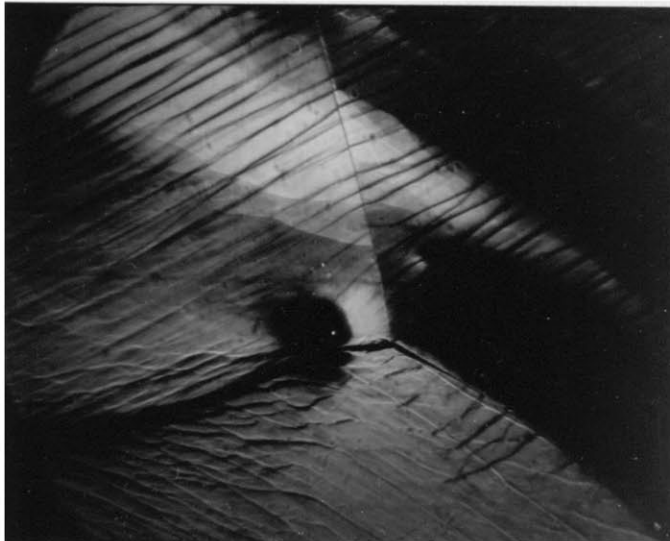
E. 162 hours after loading 400 psi. 99 hours after loading 550 psi.
