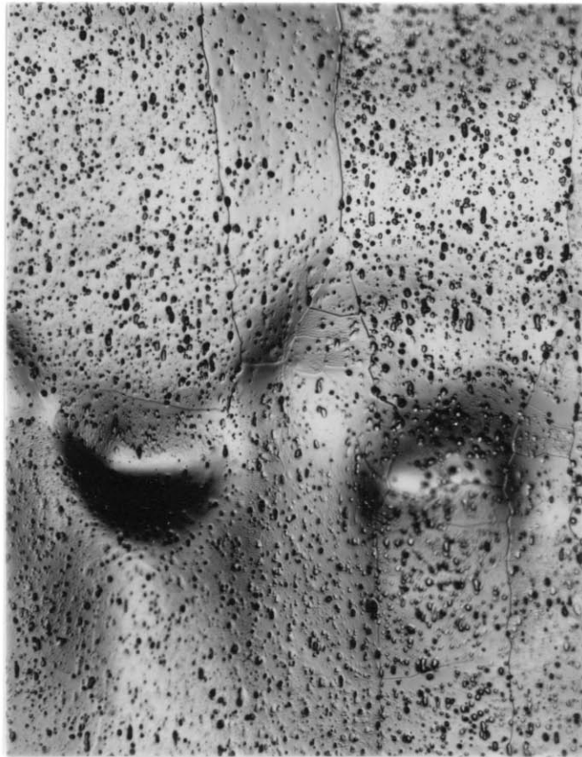
Figure 81. (Specimen 3 S -1). Repolished and etched. Sub-grain formation in 3 S aluminum. 150 X.
