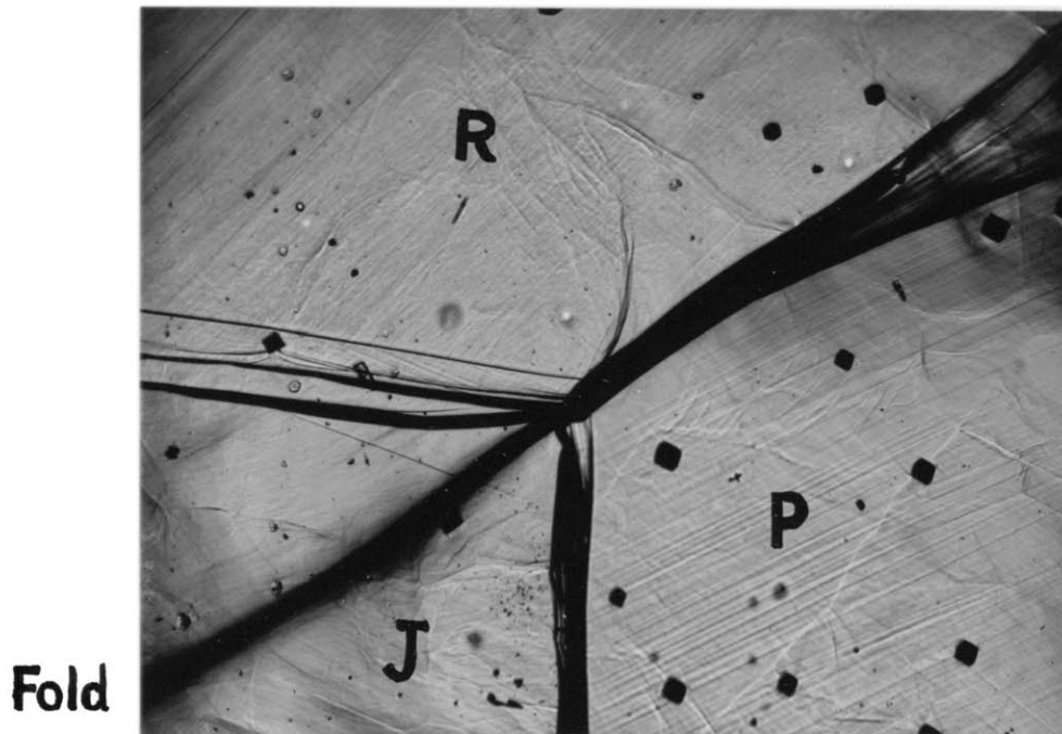
Figure 86. (Specimen P-8) front surface. Fold formation in the grain J caused by sliding of the opposite boundary. 100 X.
