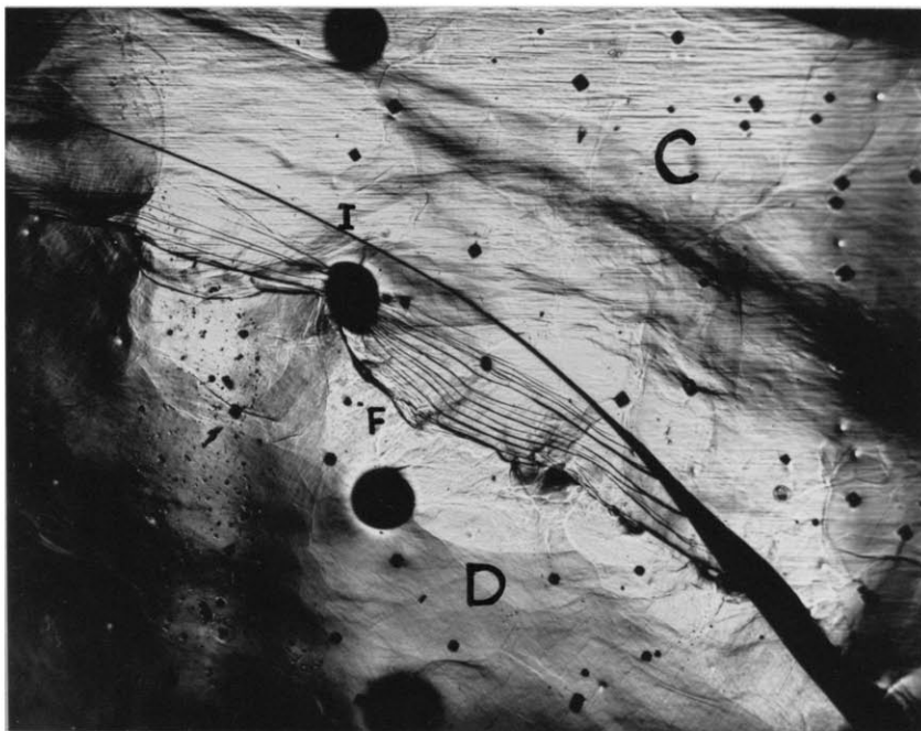
Figure 16. (Specimen P - 8, back surface). The grain boundary tended to rotate to a position perpendicular to the specimen axis. Note also the attracting effect of the needle mark on the migrating boundary. 50 X.
