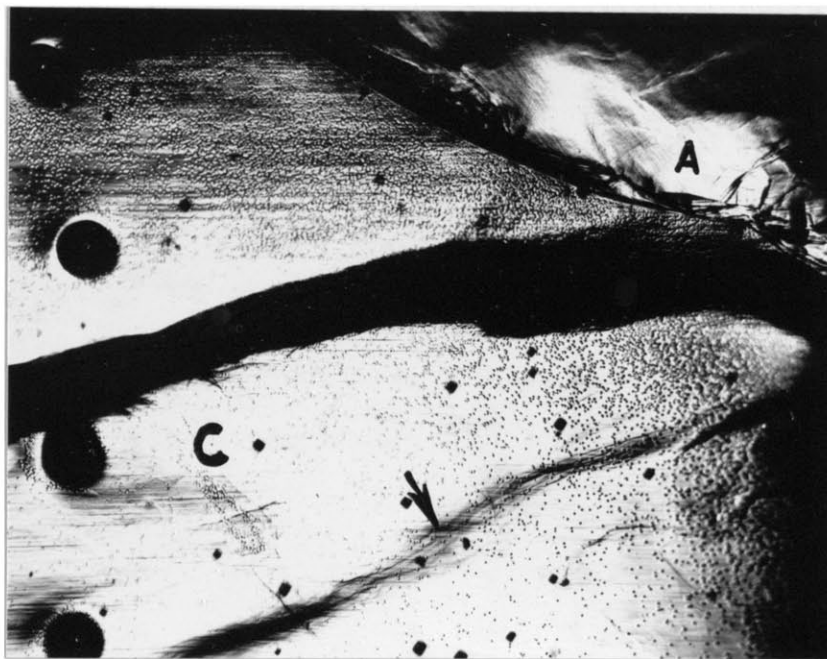
Figure 51. (Specimen P-8, front surface). A continuation of Figure 50 to the right. The upper band encountered the grain boundary at the very right edge of the specimen, the lower band encountered a grain boundary at the back surface of the specimen, incompletely developed. 50 X.
