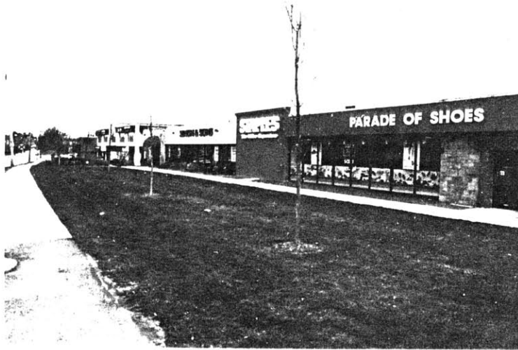
Figure 7-8: Staples has two sidewalks. The building edge sidewalk does not continue to other properties and the street edge sidewalk is inches from moving traffic (5/4/95).
