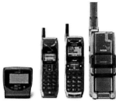
Figure 3.4 Iridium phones are currently bulkier and do not have cellular service capabilities.
