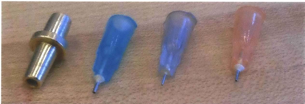
Figure 3-8: Four different size tips used with the bulb system to distribute seeds. Each tip works for different size seeds.
