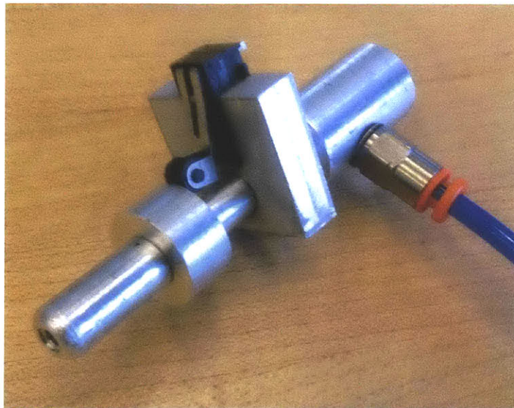
Figure 3-5: Pneumatic system that pulls a vacuum through the blue pneumatic tubing in order to take a capsule from the feeder bowl and then forces the capsule into the capsule’s carousel by changing the vacuum to outward air pressure.
