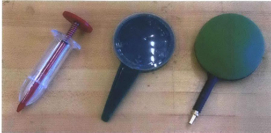
Figure 3-7: Three different systems for distributing seeds in gardens. Each was used for testing in order to determine the best system for picking up two or three seed at varying sizes. Eventually the farthest right was chosen as the best design.
