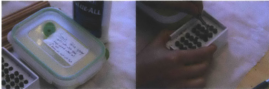
Figure 10: The glue soaked sponge in container (left); extracting a capsule with a tweezers (right)
