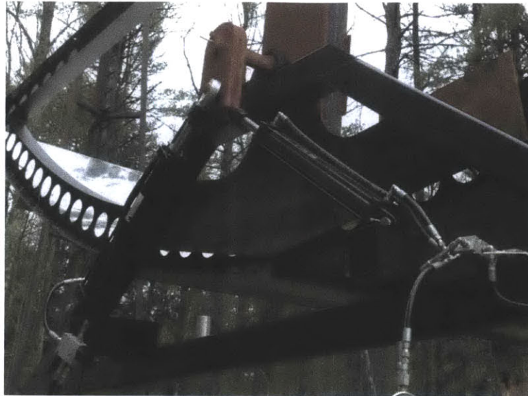
Figure 3: Existing 4 m solar trough actuation system
