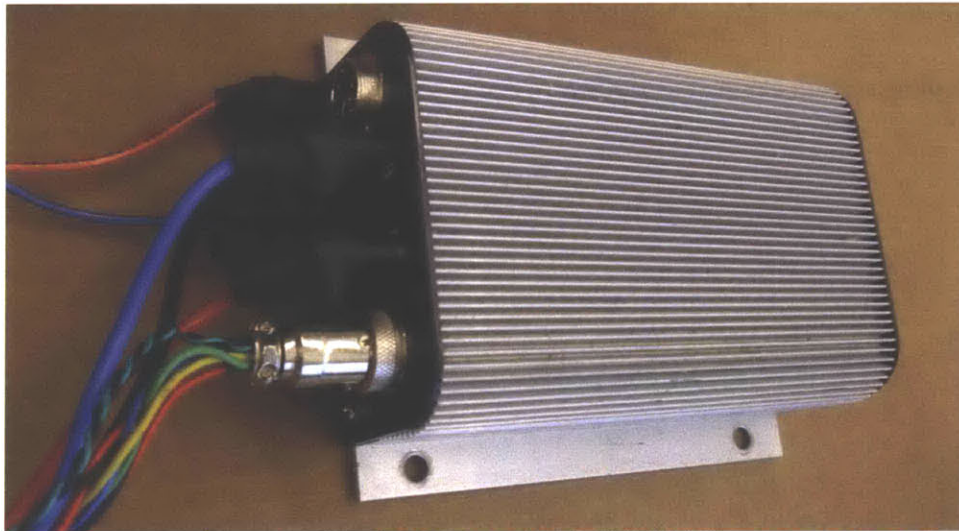
Figure 16: Motor controller box which receives power from the generator.
