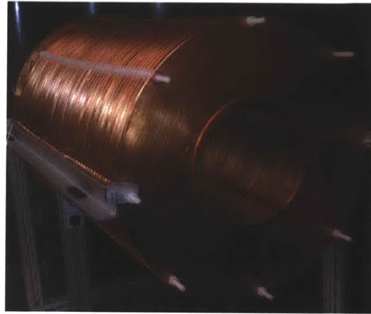
Figure 2-5: The field cage comprised of the 0.060" copper field shaping rings, cathode with viewport, and field cage maintenance stand.
