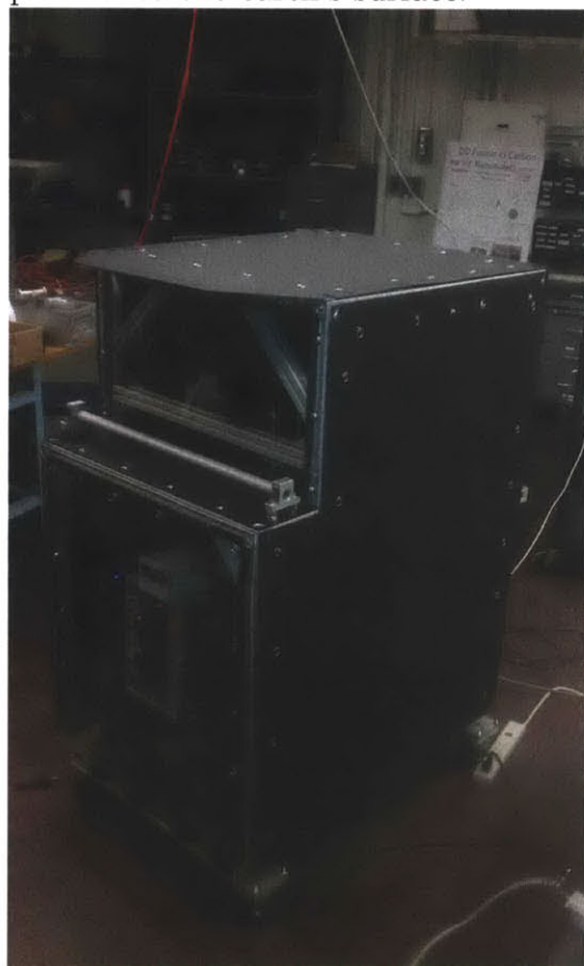
Figure 2-8: The detector configuration after the chamber was rotated and placed with amplification region parallel to the earth's surface.
