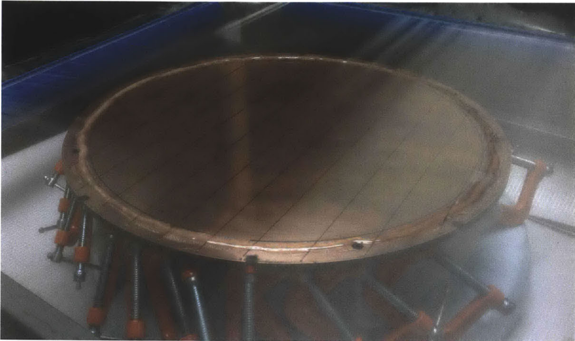
Figure 2-6: This image shows the stretched 80% transparent mesh being glued on top of the 410\mu\text{m} spacers. Additionally, the machined channels can be seen beneath the mesh around the edge of the copper clad G10.
