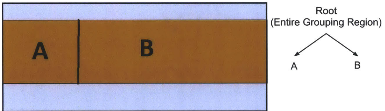
Figure 4-14: Line 1 creates Rectangles A and B. These rectangles are added as children to the root node.
