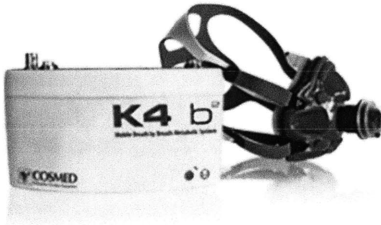
Figure 3.5 Portable COSMED K4b2 system and mask worn by subjects during experimental testing. 16
