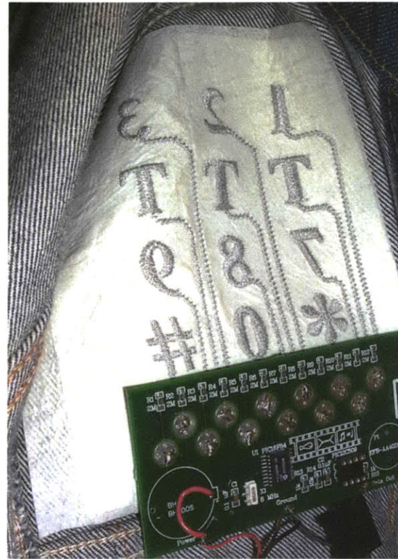
Figure 10.8 The back of the Embroidered Keypad attached to sensing electronics.
