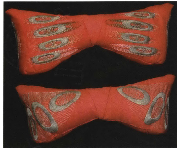
Figure 12.15 Melody Butterfly . Top, the front with four sensors. Bottom, the back with circle ground electrodes.
