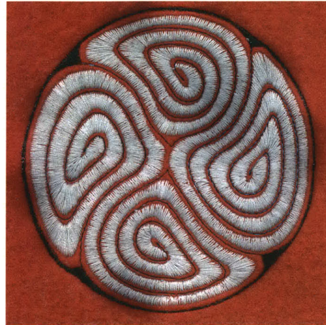
Figure 11.15 Embroidered ground electrode from the Generic Ball .
