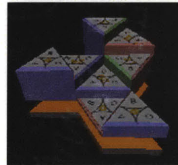
Figure 8.8 Illustration of gradient algorithm used for communication in the first generation Triangles .
