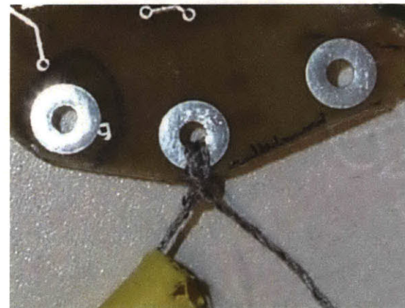
Figure 16.5 Close-up of mechanical/electrical knot with contact impedance of .2 ohms.
