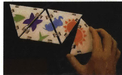
Figure 8.7 Triangles , first generation hardware, detail of connectors with sliding magnets, and image of Triangles connected.
