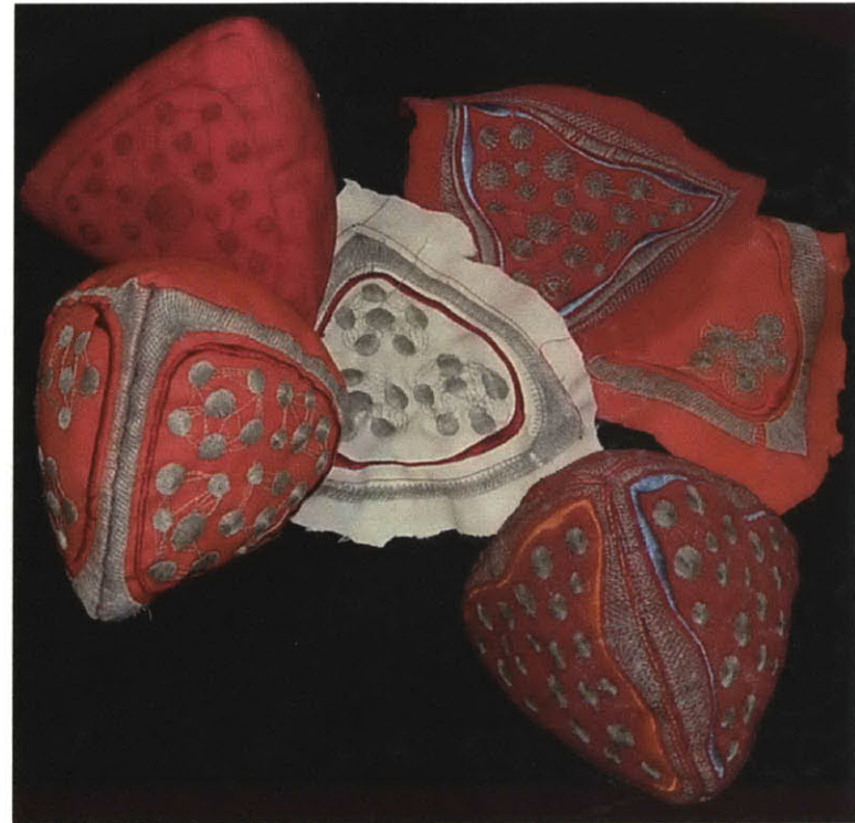
Figure 12.8 Early mock-ups for the Pyramid included a stuffed prototype with drawn sensors, and a variety of sensor and ground electrode designs.
