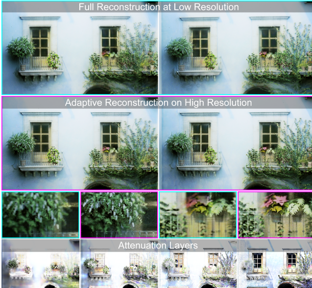
Figure 6: Photographs of two tomographic light field display prototypes. We decompose a target light field into a set of four attenuation layers (bottom), print them on transparencies and stack them using clear acrylic spacers. Two views are shown for results matching the resolution previously achieved in the literature [Wetzstein et al. 2011] (top row) and at the significantly improved resolution enabled by our adaptive framework (center row). Zoomed regions and the optimized layers are shown at the bottom.
