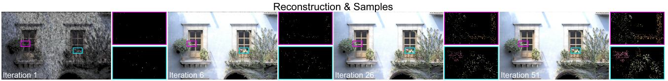
Figure 5: Adaptive tomographic light field decomposition. We show intermediate reconstructions for one view of the light field throughout the iterative algorithm. The closeups illustrate the cumulative light field samples of all previous iterations for two regions in this view. We observe that an extremely sparse set of plenoptic samples (close-ups are mostly black) is sufficient to generate high-quality reconstructions.
