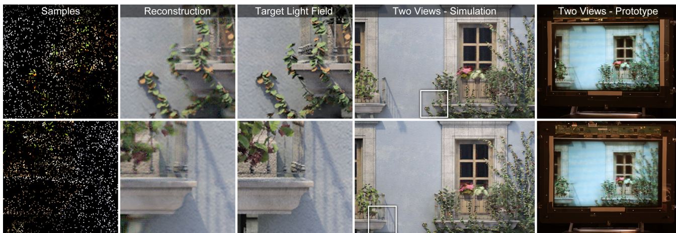
Figure 1: Adaptive light field synthesis for a dual-layer compressive display. By combining sampling, rendering, and display-specific optimization into a single framework, the proposed algorithm facilitates light field synthesis with significantly reduced computational resources. Redundancy in the light field as well as limitations of display hardware are exploited to generate high-quality reconstructions (center left column) for a high-resolution target light field of 85 \times 21 views with 840 \times 525 pixels each (center). Our adaptive reconstruction uses only 3.82% of the rays in the full target light field (left column), thus providing significant savings both during rendering and during the computation of the display parameters. The proposed framework allows for higher-resolution light fields, better 3D effects, and perceptually correct animations to be presented on emerging compressive displays (right columns).
