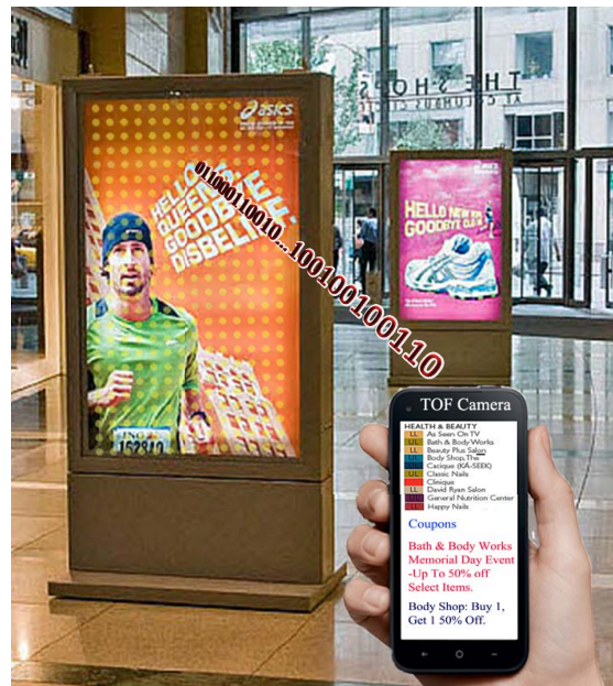
Figure 1. Concept illustration of “smart signage” for communicating to cameras in the environment with infrared LEDs that send invisible messages for communication with time-of-flight depth cameras. These cameras are increasingly more commonplace and can be expected in mobile robotics and devices. Large LEDs are shown for illustration clarity, but small infrared LEDs would be unnoticeable in a real application.
