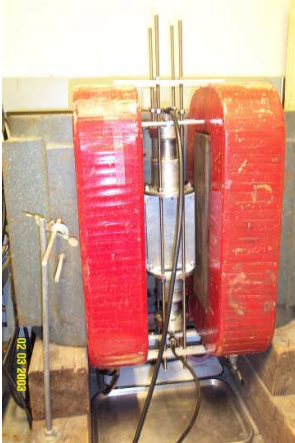
Figure 6-4: Stripline structure between the two coils (in red) (Parts B, C and D).
