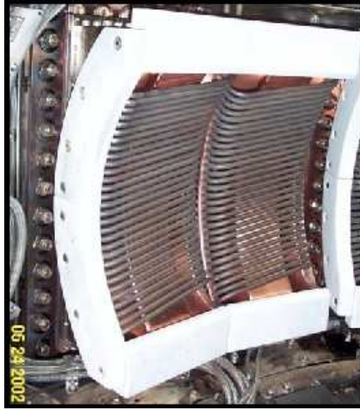
Figure 3-3: Picture of D-Antenna as installed in the vacuum vessel.
