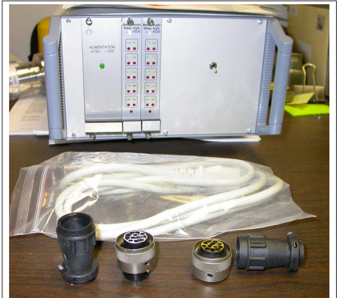
Amphenol Connectors used in the discrete level sensor
