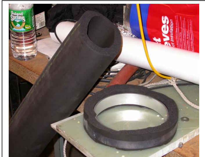
Armaflex insulation on a ring section of the vent pipe Two segments of smaller diameter pipe insulation is used for the 6 inch vent
