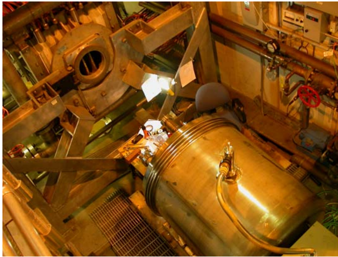
MERIT/BNL Pulsed Magnet –Inertially Cooled , LN2 or 30K He Gas Cooled Between Shots –MIT test will use only LN2
