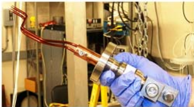
Fig. 2: Copper portion of current leads showing a) electrode clamp and zig-zag bending of the paired, 6AWG magnet wire extension, and b) thermal connection to the radiation shield and electrical connection to the HTS leads.
