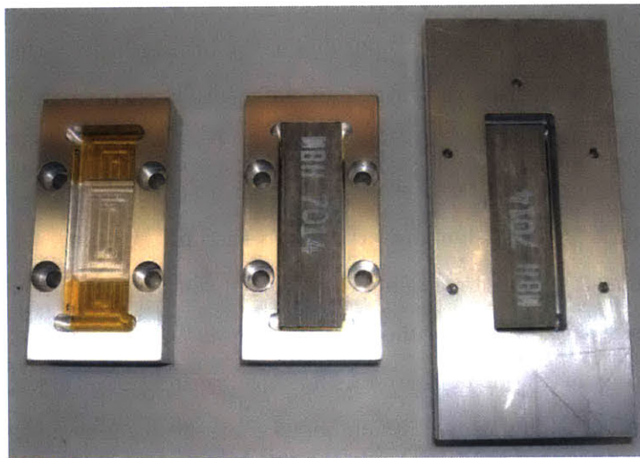
Figure 8-24: LEFT: Target housing; CENTER: Housing with I-bar in pocket; RIGHT: Mold for potting target assembly.
