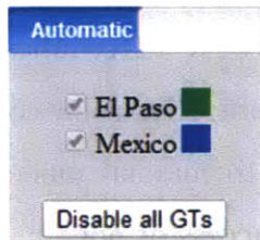
Figure 3-7: The Ground Control Station UI's interactive panel for manually overriding access control permissions. Using this panel, an operator can make the system ignore current permissions that would be implied by the state of the map interface, by changing the switch from Automatic to Manual. From there, the checklist is enabled so that the operator may manually specify which GTs should have video decryption permissions. Clicking “Disable all GTs” automatically sets the switch to manual mode, along with un-setting all GT access permissions.
