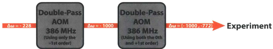
Figure 3-7: Topology of the Slower setup. First offset the whole thing by -772MHz and then using a Double-Pass AOM generate a mixed signal with the two needed outputs and send them to the experiment.
