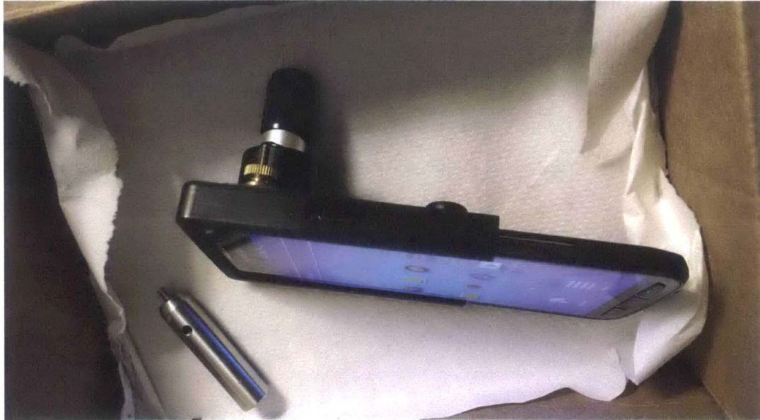
Figure 2-3: The second spectrometer prototype using a grism assembly
