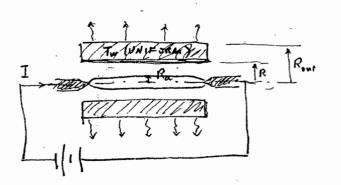
$(T_w)_{MAX}$ . Assume the constrictor is long enough that the  $\ell \sim d$ effects are negligible. There is no flow around the arc. The body of the constrictor is made of a good thermal conductor, and can be
