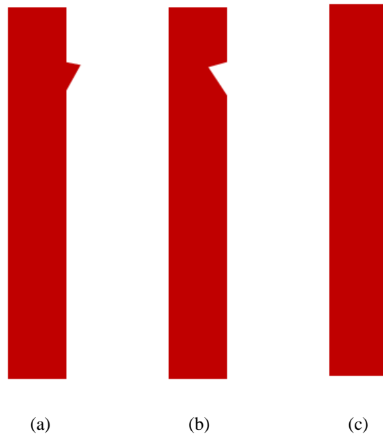
Figure 5.2: Grating tooth example: (a) Fabrication error as bulge on certain place in deformed geometry; (b) OPC on that place makes mirrored bulge, which is dent; (c) Prediction after fabrication (contour of this geometry is characterized with x and y coordinates and this is contained in contour file).
